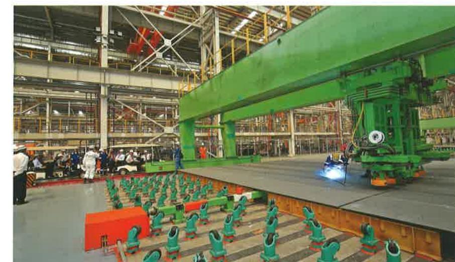
The 120,000-sqm facility included a fully-automated panel production line that delivers high quality welding precision and efficiency.
