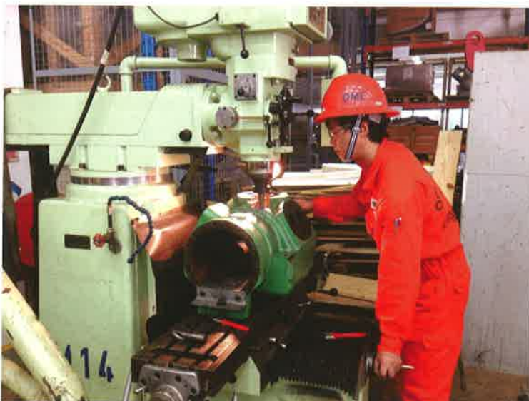
General engineering - Vertical boring of compressor housing.
