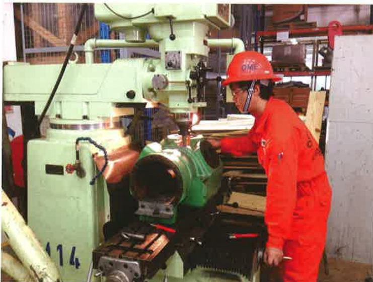
General engineering - Vertical boring of compressor housing.
