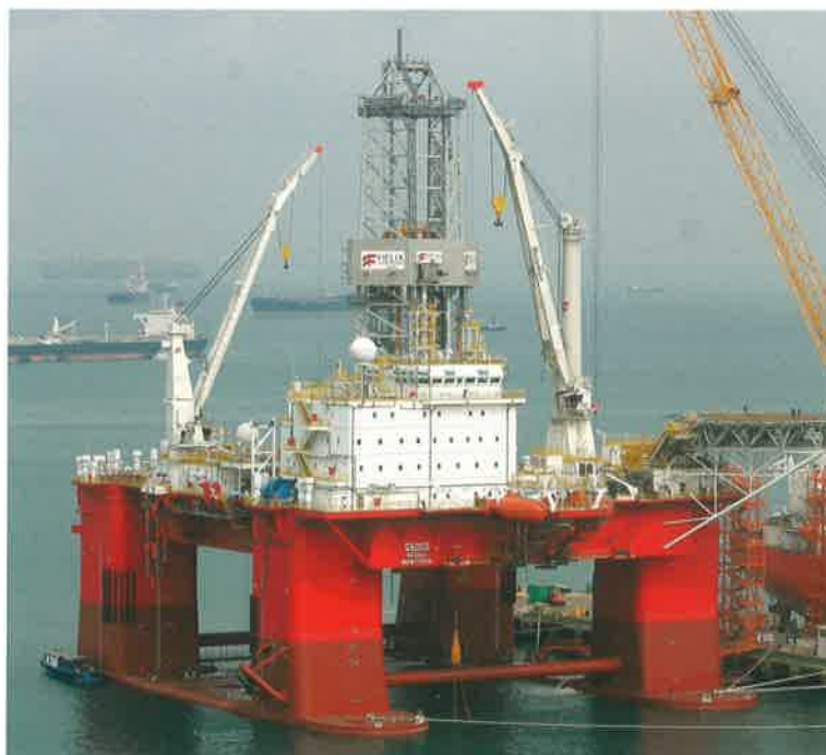
Q5000 is the first well intervention rig built by Jurong Shipyard to Helix Energy Solutions.
