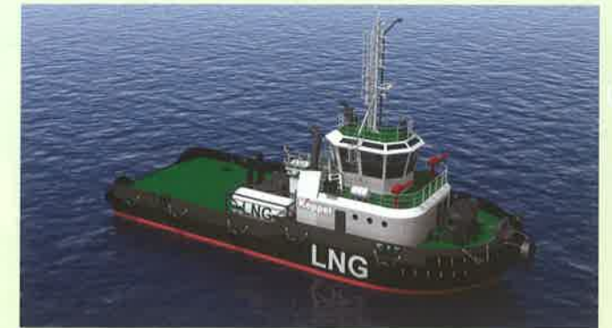
The Azimuth Stern Drive tug which can run on both LNG and diesel fuel.
