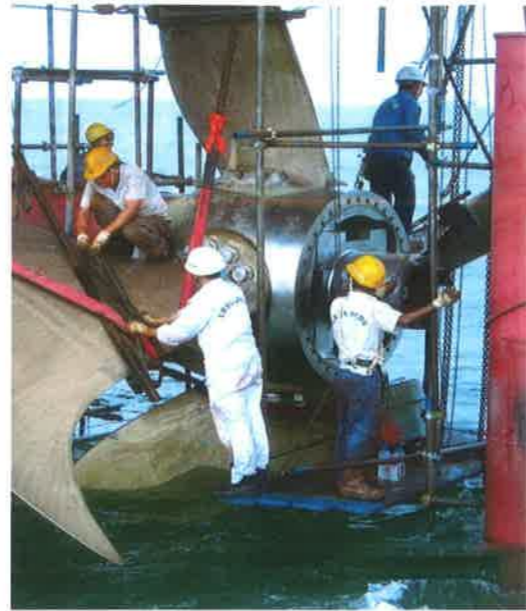
Overhauling of large CPP on Aframax tanker at anchorage.
