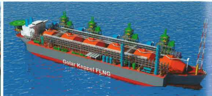
A starboard view of the Golar FLNG vessel after conversion.
