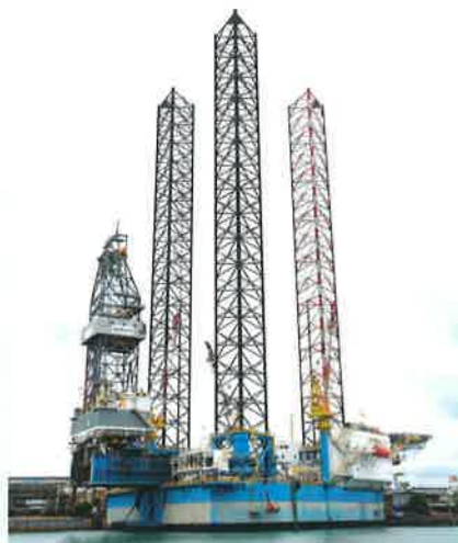
PPL Shipyard constructed Hakuryu 12 , a PC 400 design jackup rig for BOT Lease.
