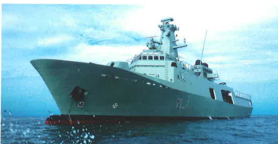
RNOV Shinas is the second of four patrol vessels designed and built by ST Marine based on its proprietary Fearless-class patrol vessel, for the Royal Navy of Oman.
