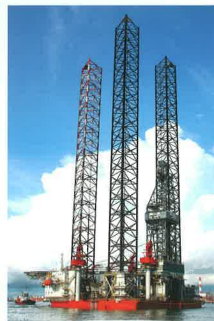
Impetus is the third PC 400 jackup rig built by PPL Shipyard for Oro Negro.
