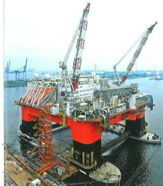
Safe Boreas , a GVA 3000E design accommodation semi-submersible built by Jurong Shipyard for Prosafe.
