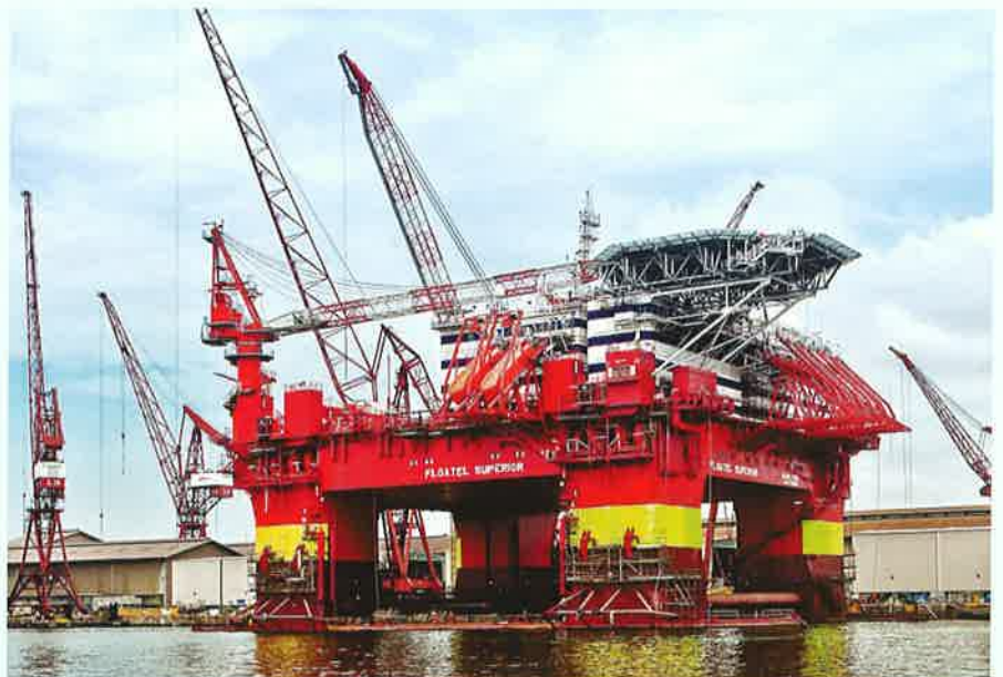
The new semi will be built to the proven Floatel Superior design, a DSS™ 20NS design developed by GustoMSC and Keppel FELS' Deepwater Technology Group.
