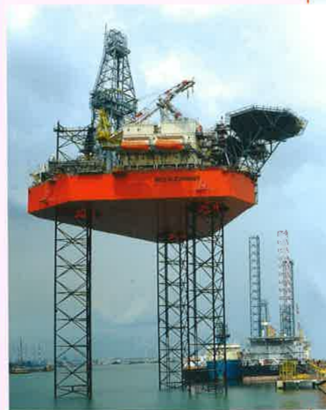
Ukraine's second jack-up rig, NEZALEZHNIIST , is built to Keppel FELS proprietary KFELS B Class design.
