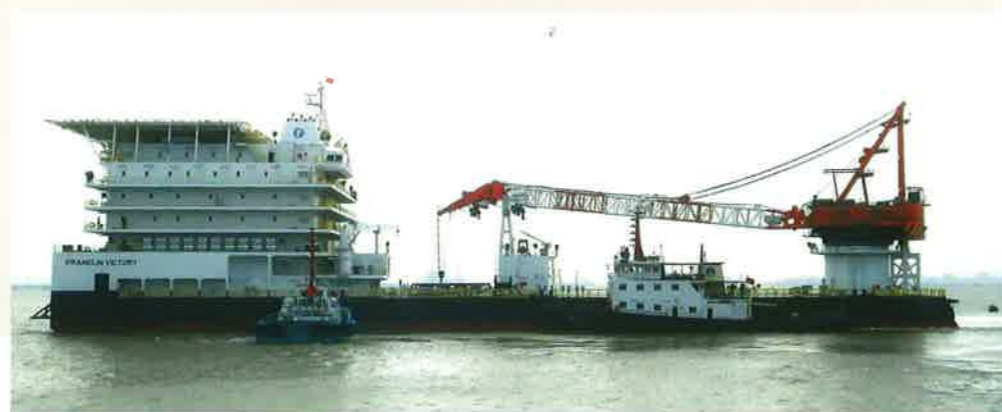
"Franklin Victory" - Franklin Offshore's new 520-tonne revolving crane construction barge is expected to enhance its ability to provide turnkey solutions for offshore permanent mooring projects.
