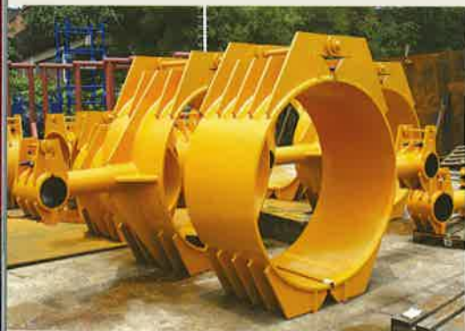
6" riser clamps for the gas lift pipeline, part of the Kodeco Project.
